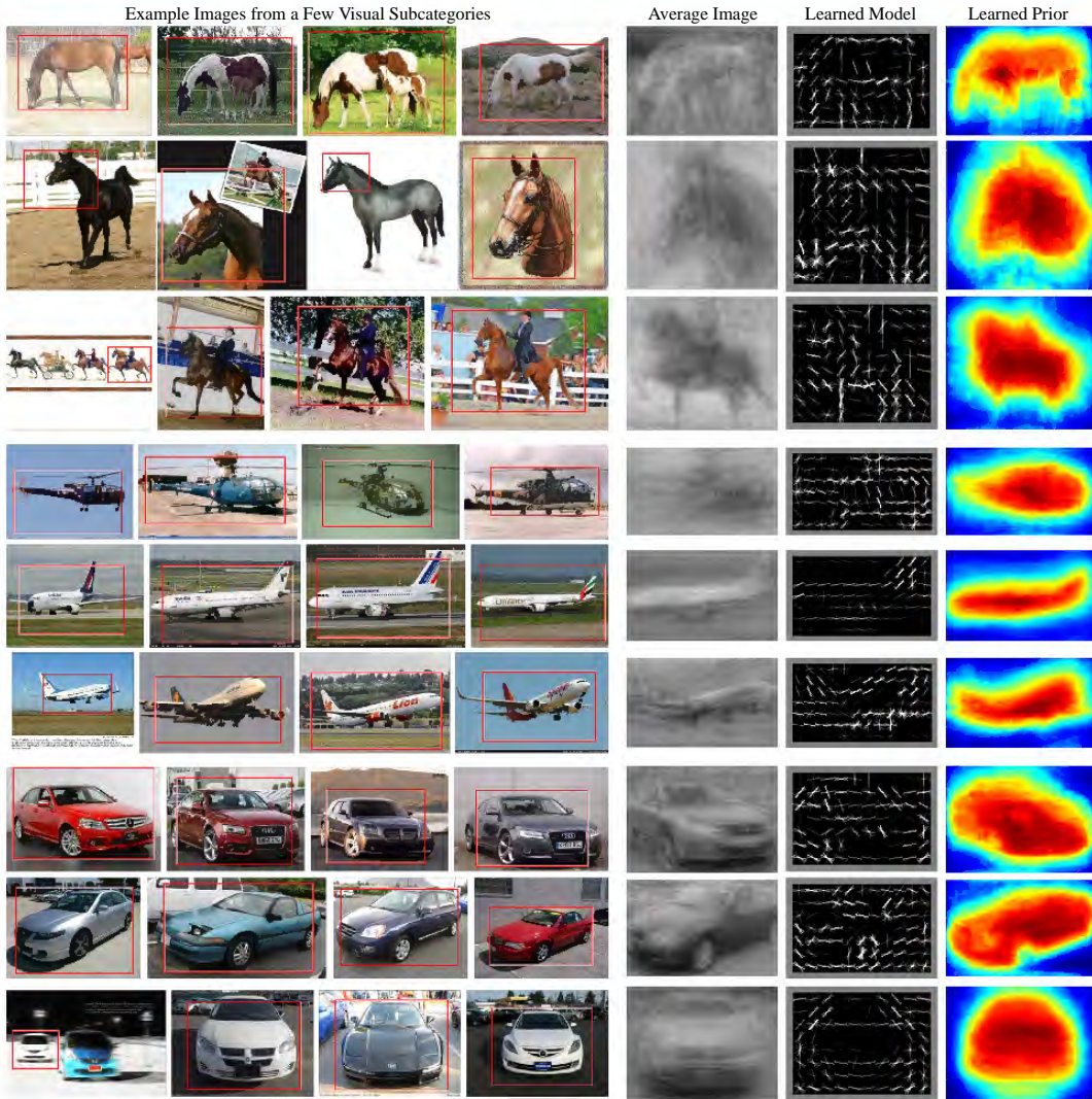
Figure 3.4: Examples of visual subcategories obtained after merging clusters. We show few instances, the average images, learned Latent SVM model and the segmentation prior for each subcategory.
