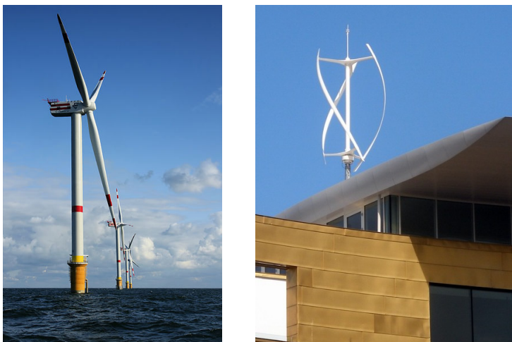
Figure 5.1: Left: horizontal axis offshore wind turbine. Right: vertical axis wind turbine. Images source: http://en.wikipedia.org/wiki/Wind_turbine .
